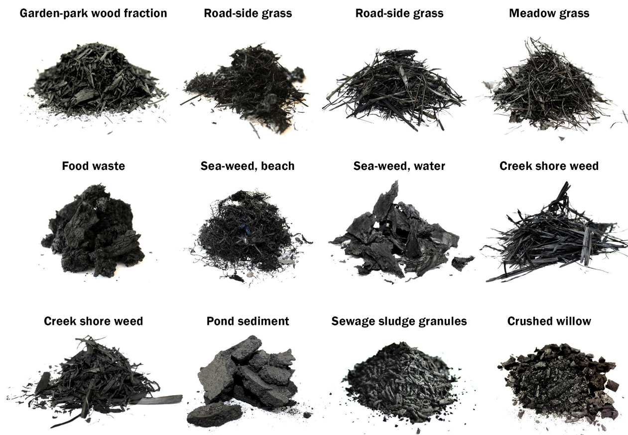
Figure 5: Pictures of biochar products from many different, Danish and Swedish biomasses 24 . By the author.
