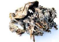
Waste water Grate material, Denmark
