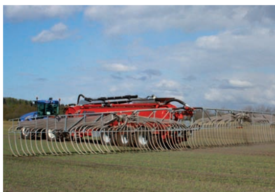
Most slurry is spread on growing winter crops in the springtime by use of large slurry tankers mounted with band laying system.
