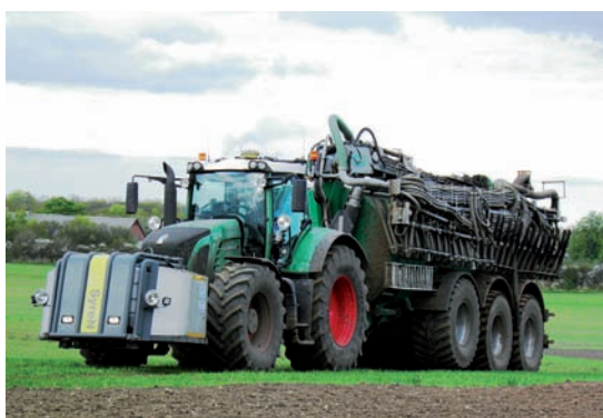
Slurry tanker with band laying system equipped with acidification system.
